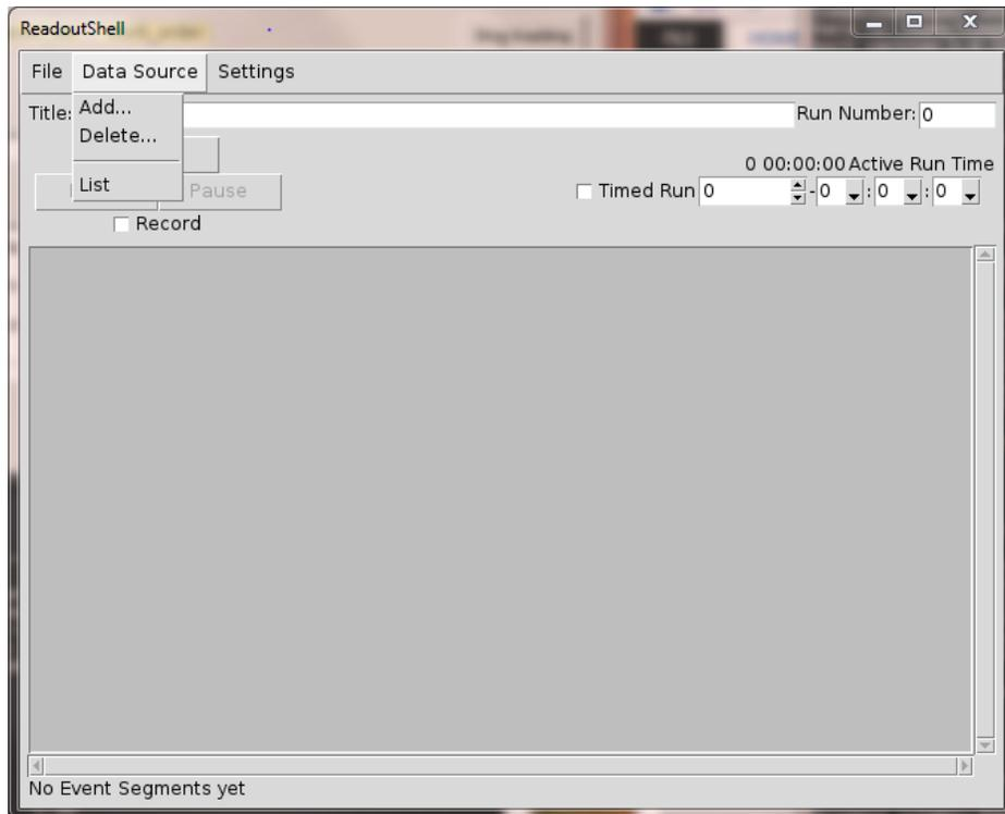
The data provider dialogue will prompt you to choose the type of data provider you are going to use. For a VMUSBReadout, CCUSBReadout, or Readout program built with the SBS Readout Framework, select SSHPipe and then press the “Ok” button.
